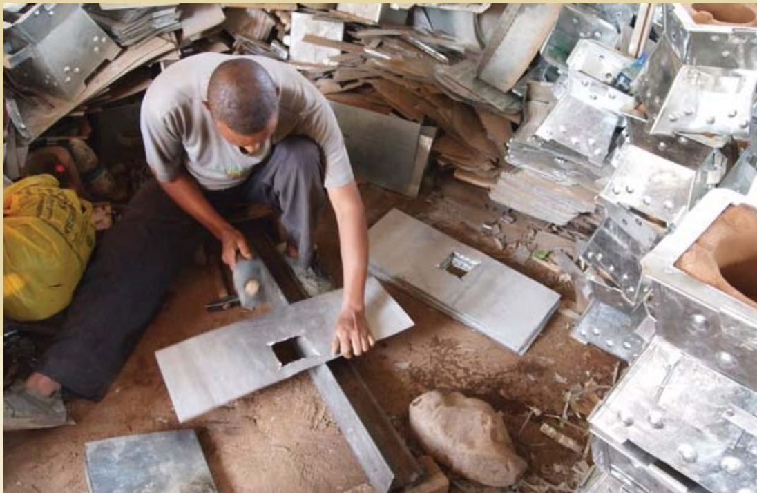
RIGHT: Local manufacturing of the Tizazu cookstove outside Addis Ababa, Ethiopia (Credit: Pepukaye Bardouille)
